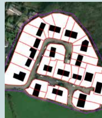
Figure 39: Diagrams illustrating the building plot coverages of 3 sample areas in the settlement area.
